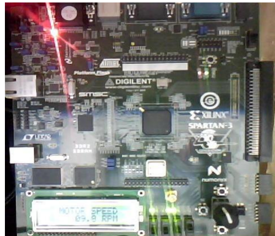
Figure 21: FLC on FPGA card.
