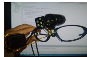
Figure 1. Proposed glass with two NIR cameras
