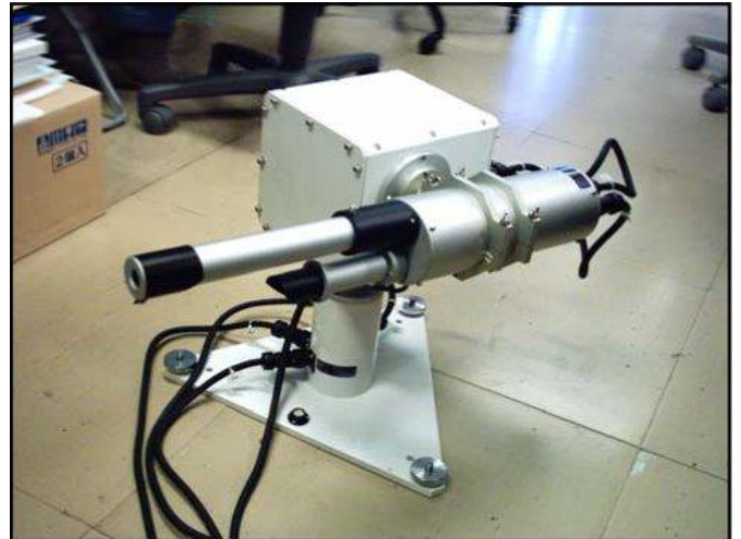
Fig. 3. Outlook of the sky radiometer manufactured by PREDE Co. Ltd. Japan
