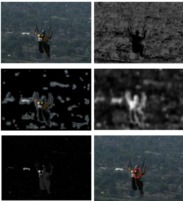
Figure 10. Testing Video 5: the illustration of one example results using our proposed model, the first left image indicates the original video, the right image shows the static saliency image; the left image on the second row shows the top-down saliency map while the right one is the motion saliency map. The third row of the left image is the fused saliency map while the right one is the attention region, red circle indicates our detected attention region by using the fusion of saliency map. The total detected frames are about 33 frames with nearly 26 frames accurately detected.
