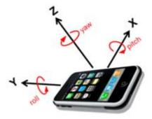
Fig. 15. Definitions of three axis coordinate and roll, pitch, and yaw rotation axis
