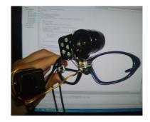
Fig. 3. Proposed glass with two NIR cameras
