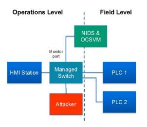
Fig. 12. Architecture of the testbed
