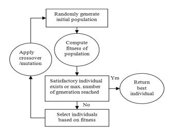
Fig. 1. Flow chart of the GP algorithm [18]
