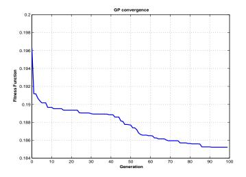
Fig. 6. Convergence of the GP evolutionary process
