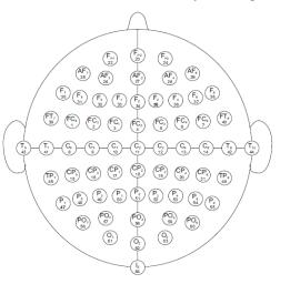
Fig. 1. Extended 10-20 international system of EEG electrodes placements
