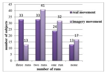
Fig. 4. Number of subjects with 100% success rate versus number of runs (EEG signal is 12-30 Hz band-pass filtered)
