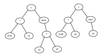
Fig. 4. Example of a Multigene Symbolic Regression Model
