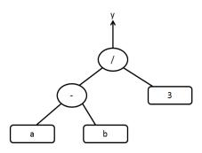
Fig. 2. Representation of a numeric expression using tree structure
