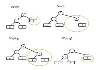
Fig. 3. A typical crossover operation
