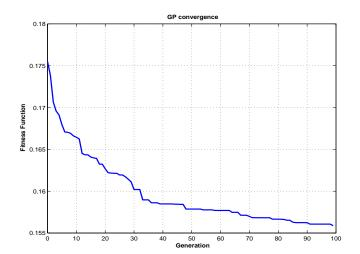
Fig. 5. Convergence of the GP evolutionary process
