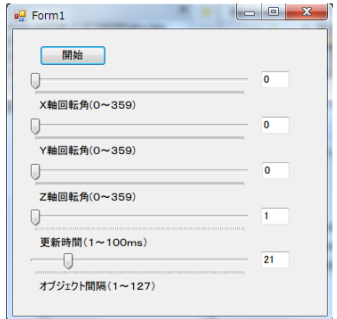
Fig. 8. Scroll slide bar for designation of parameters of 3D object image representations (the slide ruler is for the rotation angle in x axis followed by y and z axis and refresh cycle of the time interval of display as well as object frame interval ranges from 1 to 127
