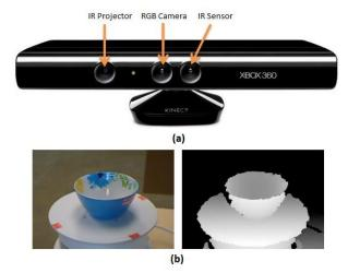
Fig. 1. Illustration of 3D camera and RGB-D data: a) Microsoft Kinect Device; b) an object example of RGB-D data is captured by Kinect
