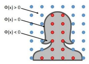
Fig. 4. Illustration of SDF for object's surface
