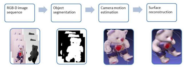
Fig. 2. Flowchart of 3D object reconstruction system in RGB-D data
