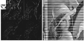
(c) MRA image with secret image (d) Reconstructed image (Level 3) Figure 1: Resultant images of wavelet based MRA which contains the secret image of Mandrill (left bottom), LL (left top), LH (right top), and HH (right bottom) as well as reconstructed image (circulation image) which contains embedded secret image
