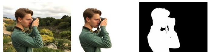
Fig. 3. Output of the framework consisting of RGB Image, extracted frontal area and alpha matte (From left to right).
