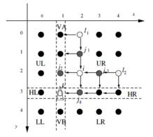
Fig. 4. Divided Subareas, and Data Flows Received and Transmitted at Node i [9]
