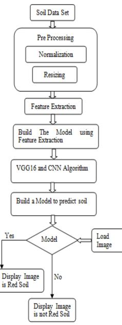
Fig. 2. Detailed Soil Classification Architecture.
