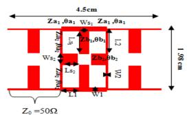
Fig. 7. Design of the T model branche line coupler with a low impedance
