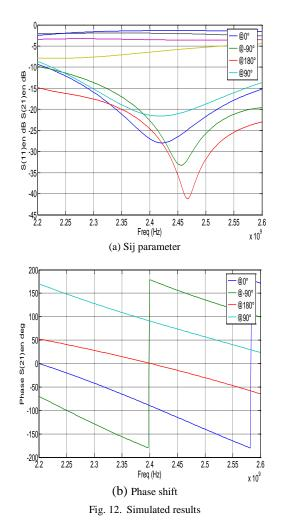
We obtain the same performance of the conventional PS, but we notice an increase of the insertion losses especially for the phase  $180^{\circ}$ . The phase shift between the four states is equal to  $90^{\circ}$  in the centre frequency and we obtain a good adaptation.
