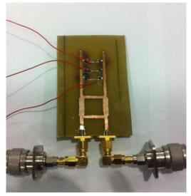
Fig. 3. Fabricated 2-bits PS
