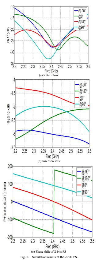
Simulation results of the four phases show a return loss better than -15 dB, an insertion loss less than -3dB over 2- 2.6 GHz. The phase shift is equal to  $90^{\circ}$  with error of  $0.5^{\circ}$  in the centre frequency. The objective of the next paragraph is to validate our simulation through a realised experimentation setup.
